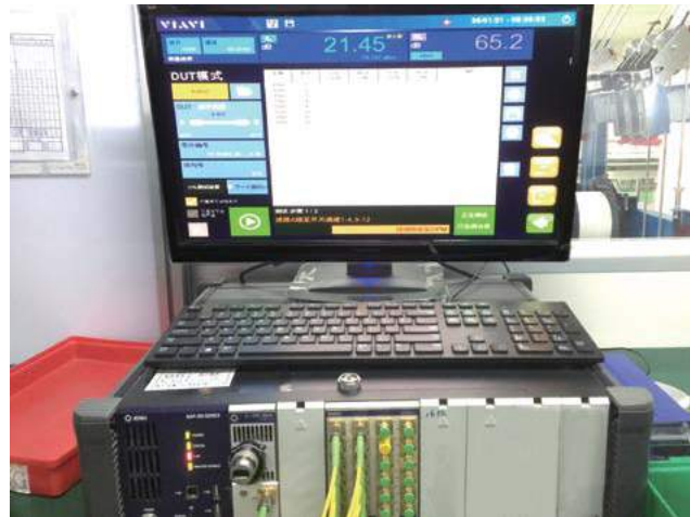
JDSU 32 port Single-mode Insertion Loss & Return Loss
