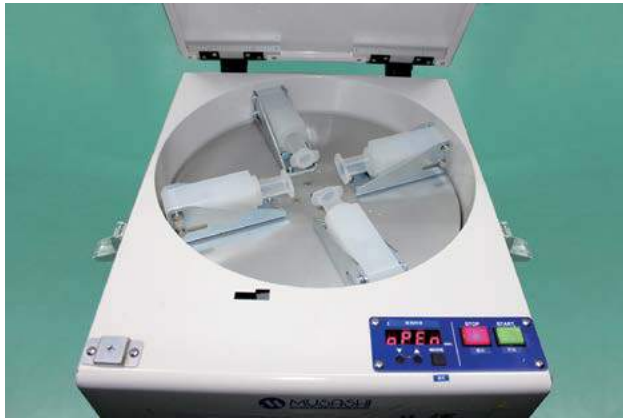
Centrifugal degassing: Remove bubbles from the syringe
