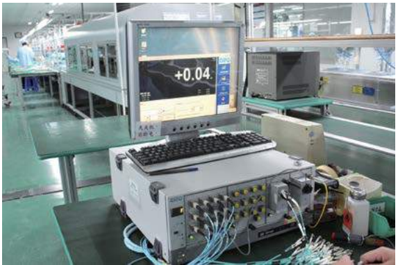
EXFO 24 port Multimode Insertion Loss & Return Loss
